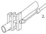
2. Note: After the tool is loosened, you may rotate the squeeze-off tool 90° and reapply pressure to round out the pipe and make installing the support clamp easier. Remove the squeeze-off tool.
