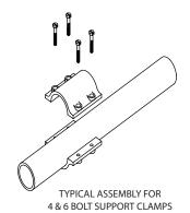
3. Place top and bottom halves of support clamp over squeezed area. Install bolts and tighten evenly until flanges meet.
